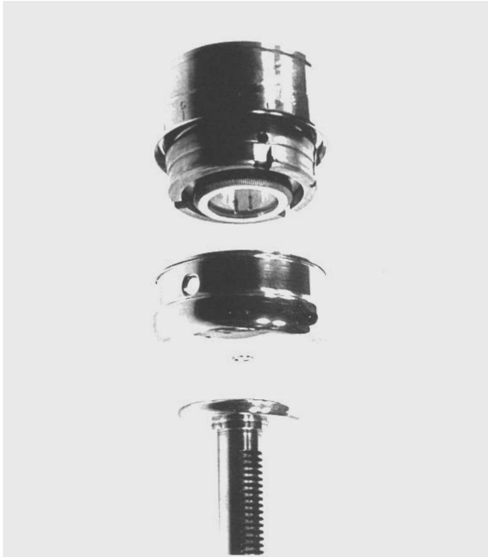
Figure 5.2. The three major parts of a thermionic gun, from top to bottom: the cathode, the Wehnelt cylinder, and the anode, shown separated. The Wehnelt screws onto the cathode (filament) support and both are attached to the high-tension cable which contains power supplies for heating the filament and biasing the Wehnelt. The anode sits just below the Wehnelt, in the top of the TEM column.
