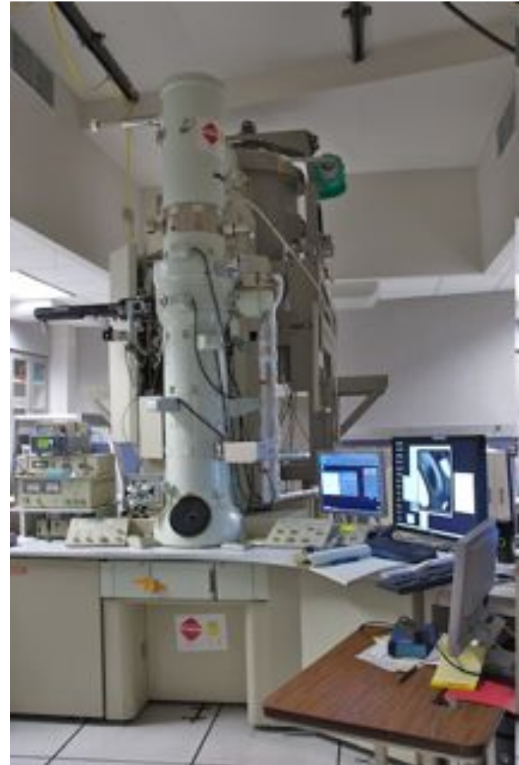
JEOL3200FSC: 300 kV, N 2 , Energy filter ~1500 micrographs, 50k mag 1 exposure, on film, Nikon scanner
