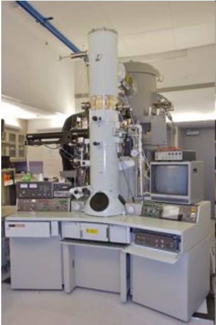
JEOL3000SFF: 300 kV, Helium ~3000 micrographs, 60k mag 1 exposure, on film, Nikon scanner,
